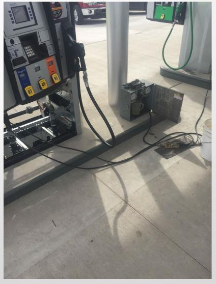
LDT-890 testing through the shear valve
