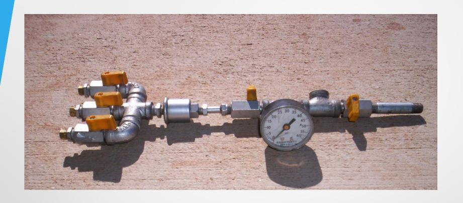
An example of fixed orifice test equipment that does not meet the quality standard. Estabrook's Leak Detector Tester
