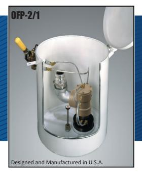
Meets Uniform Fire Code (August, 1994), Article 79 Flammable and Compustible Liquids: "shut off the flow into the tank at 90% capacity" and "means shall be provided to empty the fill hose into the tank after the automatic shut-off device is activated." Installation instructions provide plumbing details and optional parts to complete this style of installation, additional part OFP-1030 is required.
