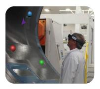
The delivered system consists of spheres locating the potential defects identified by the composite layering robot. Through a movable floating interface, the technician can then quickly inspect the location, and update its repair status in real-time.
