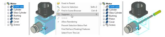
**[G]** – *Ghost* (a transparent hidden "ghost model") can be applied to one or more Assemblies or Parts. Is meant to be used as a reference model in the 3D scene, where it cannot be selected or modified. With a setting applied it can be allowed to use for snap-to referencing with handles or the TriBall.
