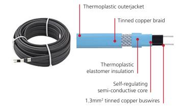
Self-regulating heat cable, also known as self-limiting heat cable or heating tape, automatically varies its power output as the pipe or ambient temperature changes.
