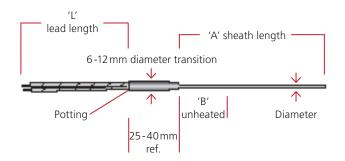
Cable heaters are a versatile heating element and are often used as an emergency replacement for mica bands.
