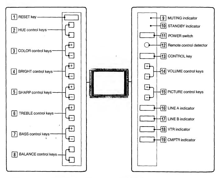
• Press CONTROL key after power is turned on to light the control keys or indicators.
