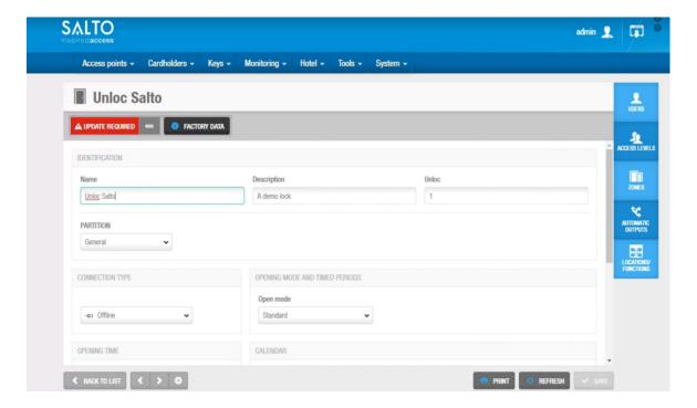
Each lock that should be Unloc compatible needs to set the field "Unloc" to the lock type id corresponding to the lock that is installed. The list of available lock
