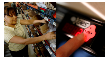
4. Item is picked; picker presses "OK" to verify completion of task
