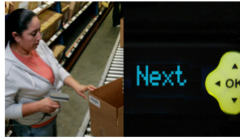
2. Picker inducts order by scanning tag or pushing "OK" at "Next" prompt
