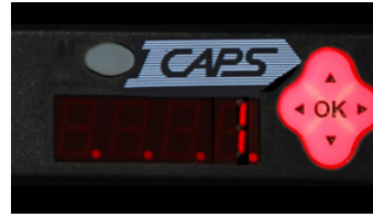
3. Lighted display indicates item and quantity to be picked
