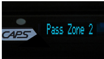
5. Zone Controller beeps and indicates where the order goes next
