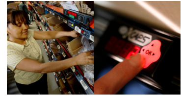
4. Item is picked; picker presses "OK" to verify completion of task
