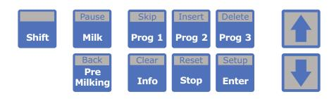
The keypad is constructed from a tough membrane overlaying individual key switches. This is a proven, reliable construction which will last for many years provided it is cleaned only with warm soapy water and not hosed down at high pressure.
