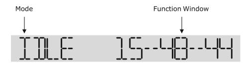
The display has two areas. The Mode area shows the current mode - either Idle when neither milking or washing, Milk when in Milking Mode or PRE, PG1, PG2 or PG3 when in Washing Mode. The Function area shows where the control is in Wash Mode or displays the time in Milking or Idle Modes.
