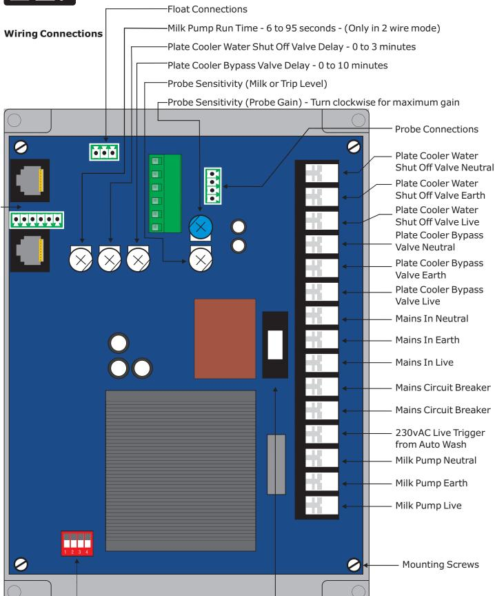
Mounting screws have plastic washers between printed circuit board (PCB) and lid mount. If not installed, the buttons will not function.
