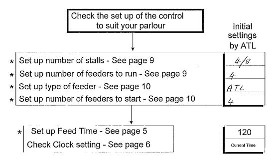
\* NOTE: When running these sub routines - press RESET to leave the value as it is or type in new value and press ENTER
