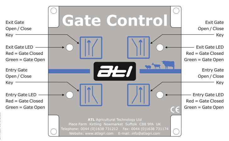
NB - Whether the gate LEDs show red for gate closed and green for gate open is dependent upon how the solenoid(s) are connected to the outputs on the printed circuit board.
