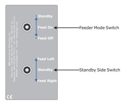
To use the standby feeding mode, switch the feeder mode switch to standby and then flick the standby side switch to either the left or the right depending upon which side you would like to feed. This will then deliver a calibrated ration of 1 unit of feed to be delivered through all the feeders on the parlour side selected. Flick the switch to deliver as many units of feed as required.
