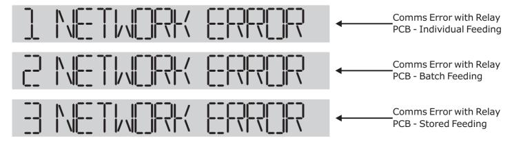
Error Messages - During Setup - In all cases check network connection to relay PCB.
