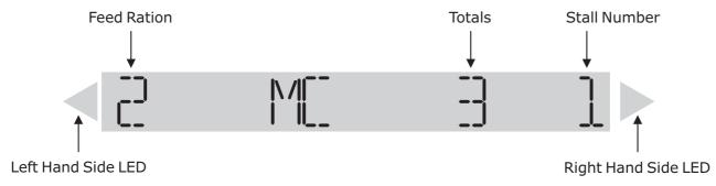
The display area comprises five windows. The Ration window shows the ration that has been keyed. The Totals window shows the feed dispensed or cows fed during the current milking, the total feed consumed to date and various values during the setup procedure.
