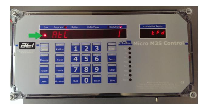
10. Check the program light is on, if not run subroutine 638 (Press Shift and Enter at the same time, then type 6, 3 then 8, then press enter).
