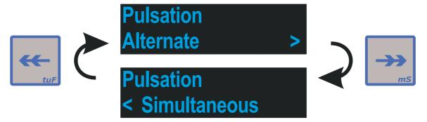
When the correct setting is selected, press the Milk key to store the data. The pulsation output invert function is now displayed.
