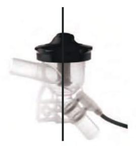
The ACR sensor should be installed so that it is aligned correctly. The vertical alignment should match the picture shown above. If the sensor is not installed in this alignment, it will not function correctly.
