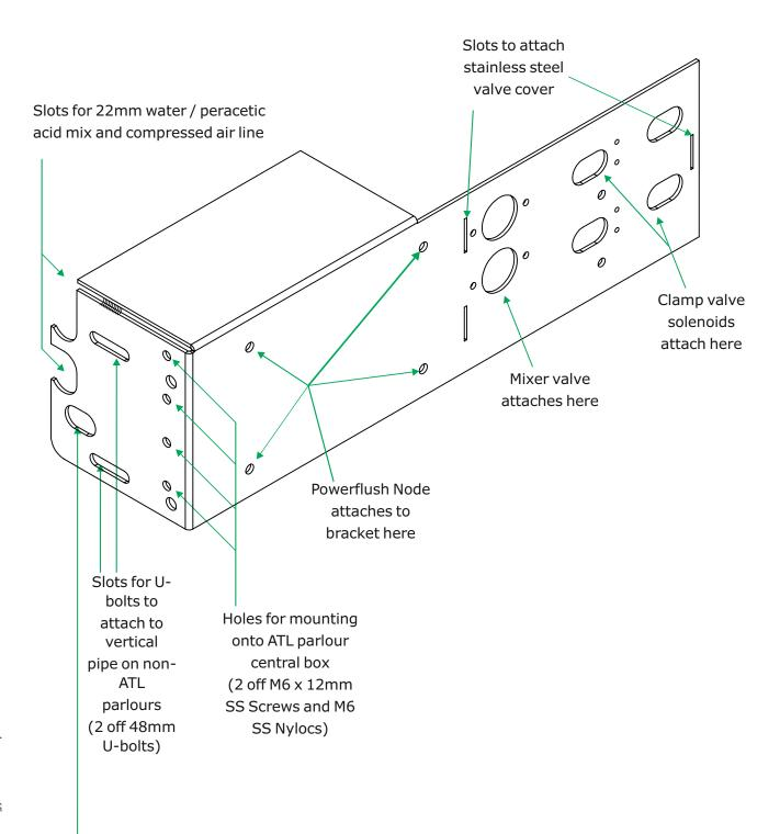
Slot for 12mm high pressure compressed air line for clamp and safety valves
