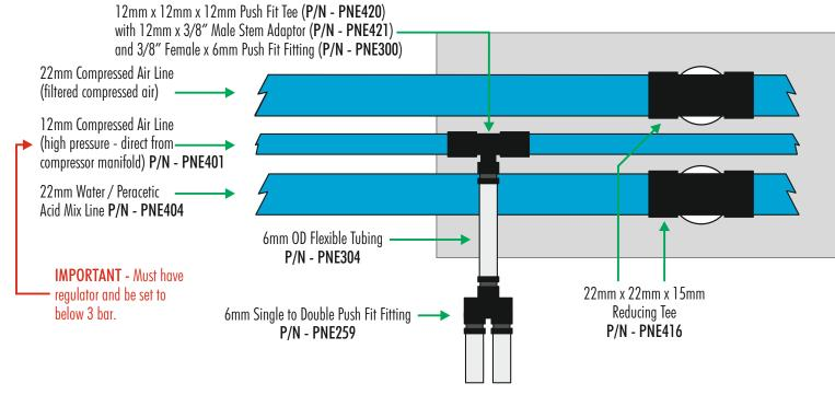
**IMPORTANT -** The 22mm compressed air line must use filtered (clean, dry and oil free) compressed air. If unfiltered compressed air is used, ATL is not responsible for any issues this may cause.
