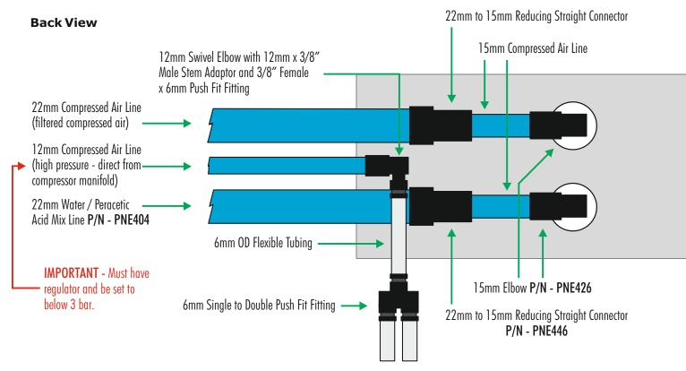
IMPORTANT - The 22mm compressed air line must use filtered (clean, dry and oil free) compressed air. If unfiltered compressed air is used, ATL is not responsible for any issues this may cause.
