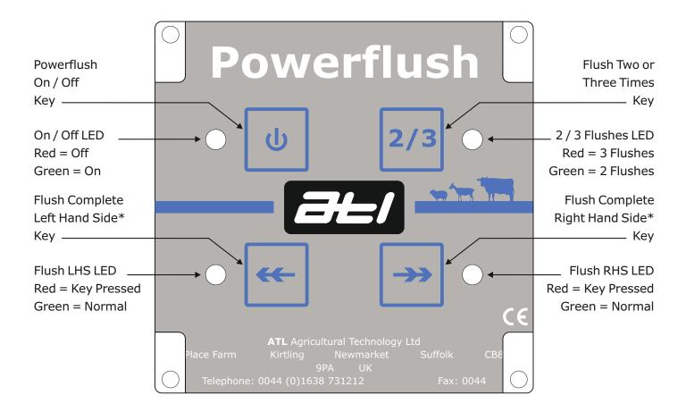
\* On a swingover parlour, either the flush complete left hand side key or flush complete right hand side key can be pressed to flush all the units. This is set from the Master PCB in the power supply.
