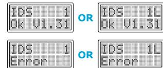
The information displayed on the LCD will display depend upon whether the system is setup as a swingover (left graphic) or doubled up (right graphic) parlour.
