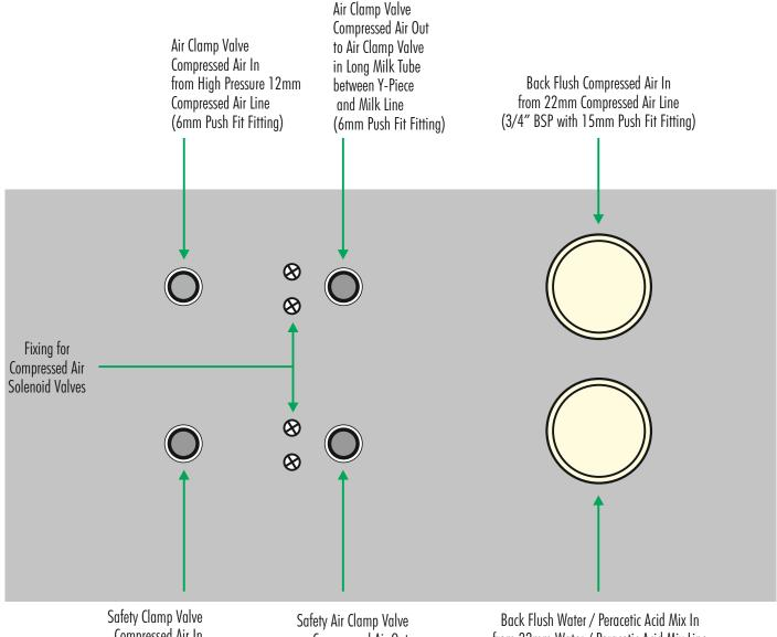
Safety Clamp Valve Compressed Air In from High Pressure 12mm Compressed Air Line (6mm Push Fit Fitting) Safety Air Clamp Valve Compressed Air Out to Safety Air Clamp Valve in Flush Line Tube between Y-Piece and Mixer Valve (6mm Push Fit Fitting)
