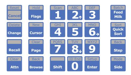
The keypad is constructed from a tough membrane overlaying individual key switches. This is a proven, reliable construction which will last for many years provided it is cleaned only with warm soapy water and not hosed down at high pressure.
