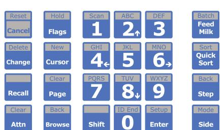
Press any of the keys and the display will show the key pressed. If a key does not show on the display, the key is more than likely faulty. The display below shows what happens if the Enter key is pressed.
