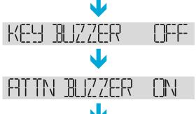
Key Buzzer: This setting controls whether the control beeps when a key is pressed.
