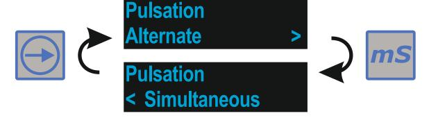
When the correct setting is selected, press the Milk key to store the data. The pulsation output invert function is now displayed.
