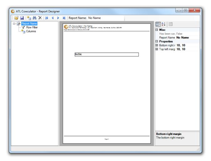
The main menu tool bar at the top of the dialog allows the user to add, remove and edit columns and search filters attached to the report. The tool bar buttons are described below;
