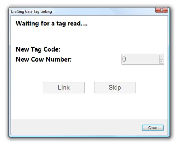
Here it is shown waiting for a tag to be read by the system. When a tag code is received, it will be displayed, the dialog will then wait for the user to enter an animal number. Any tags read whilst the user is entering a tag number will be remembered and displayed consecutively.
