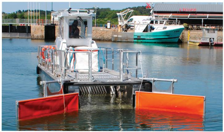
The WasteCleaner 92 is a clean up vessel with a unique and innovative technology for collecting solid and liquid waste including hydrocarbons.
