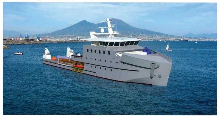
SpillCleaner 650 is a multipurpose and clean-up vessel with a unique and innovative technology for collecting solid and liquid floating waste including hydrocarbons. It is fully automated, all controls for pollution containment are carried out from the wheelhouse. The ship is an offshore vessel capable of staying at sea for several weeks in multi-mission.
