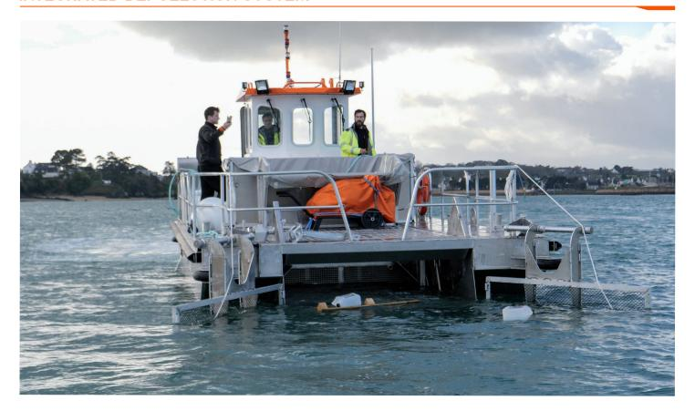
The MultiCleaner 100 is a multipurpose and clean-up vessel with a unique and innovative technology for collecting solid and liquid floating waste including hydrocarbons.
