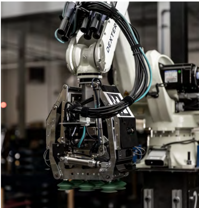
CLOSED GRIPPER TO PICK INDIVIDUAL ITEMS
