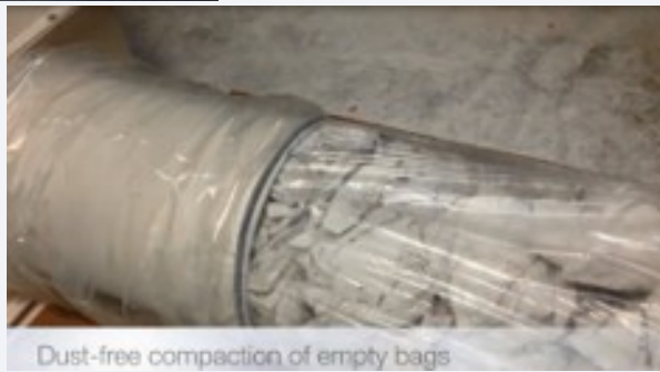
Dust-free compaction of empty bags
