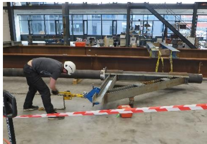
Photos: Factory Acceptance Test of winch and davit structure
