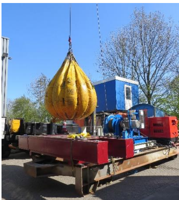
Photos: Factory Acceptance Test of winch and davit structure
