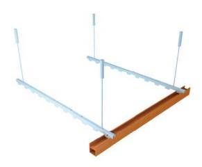
2. Install the first TH9050HD profile to the substructure.
