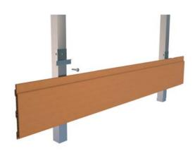
4. Insert the second row of clips to lock the plank.
