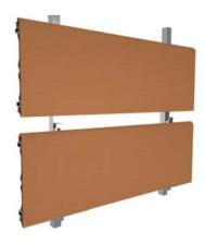
**6.** Repeat as described from step 3 up to the top to complete the cladding.
