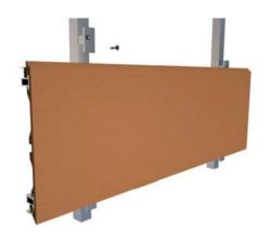
4. Insert the second row of clips to lock the plank.
