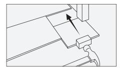
7. The final row must be a minimum 40mm in width. Glue the last rows end joins with PVA glue if not able to side-tap.
