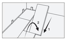
Always tap the long join with a tapping block to ensure complete engagement. Never strike the floor directly as this will damage the locking system – always use a block.
