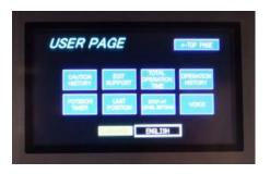
Easy to read, high-contrast, color touch screen for backup control and over 40 alert codes that can be visualized for service diagnostics.
