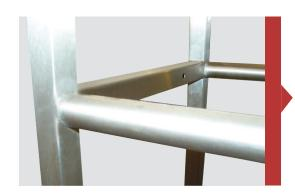
Special tubular frame construction. TipTrak™ Open Frame/Tubular units are made using square/round tubing to minimize ledges that can catch or trap product. Equipment sections bolt together for easy installation. Welded bolt sleeves eliminate the possibility of water collection inside the frame. Casing type (enclosed) frames are also available with special access doors to accommodate wash-down cleaning.
