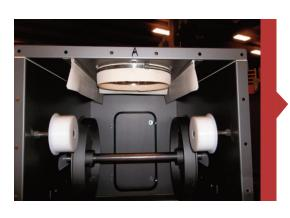
Special inlet design. UniTrak uses a custom round inlet for a better sealed connection to your infeed equipment. Includes the addition of an internal natural rubber tube that directs the product and fines into the buckets.
