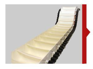
**Rubber** *beltchain*. The rubber *beltchain* is the very heart and soul of TipTrak<sup>™</sup> bucket conveyors. Consisting of super-tough elastomer molded around and bonded to a core of multiple strands of stainless steel aircraft cables, the TipTrak<sup>™</sup> *beltchain* provides years of reliable, trouble-free service. For cold applications, we can supply a TipTrak<sup>™</sup> *beltchain* made from an elastomer specially formulated to provide assured startup and operation.
