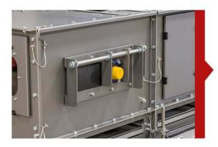
**Equipment frames.** Low temperatures may cause condensation to deposit on the conveyor frame. Since condensation has the potential to cause corrosion, TipTrak<sup>™</sup> conveyors can be supplied in either stainless steel or carbon steel with a corrosion-inhibiting paint finish.
