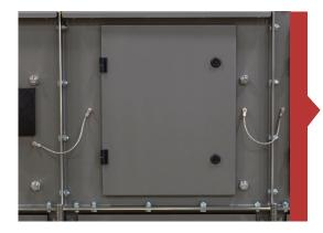
**Ground studs and grounding wire.** The entire TipTrak<sup>™</sup> is grounded via welded grounding studs and ground straps on each panel of the entire frame to ensure a fully conductive path to ground, or "earthing".
