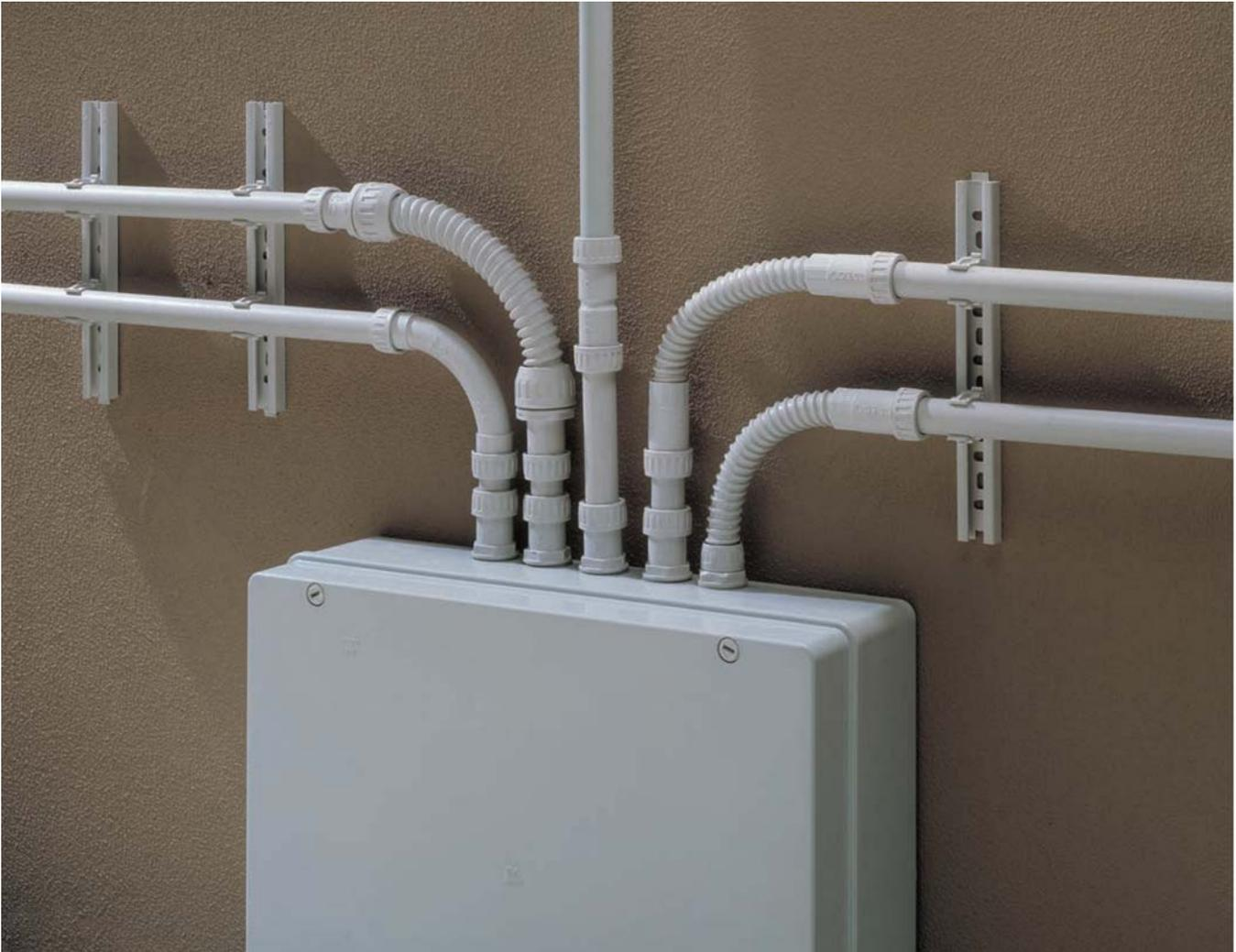
EC conduit fitting system covers all installation needs: watertight rigid conduit-box joint, couplings, 90° bends, rigid conduit-spiral conduit joints to connect two conduits with same or different diameters.
