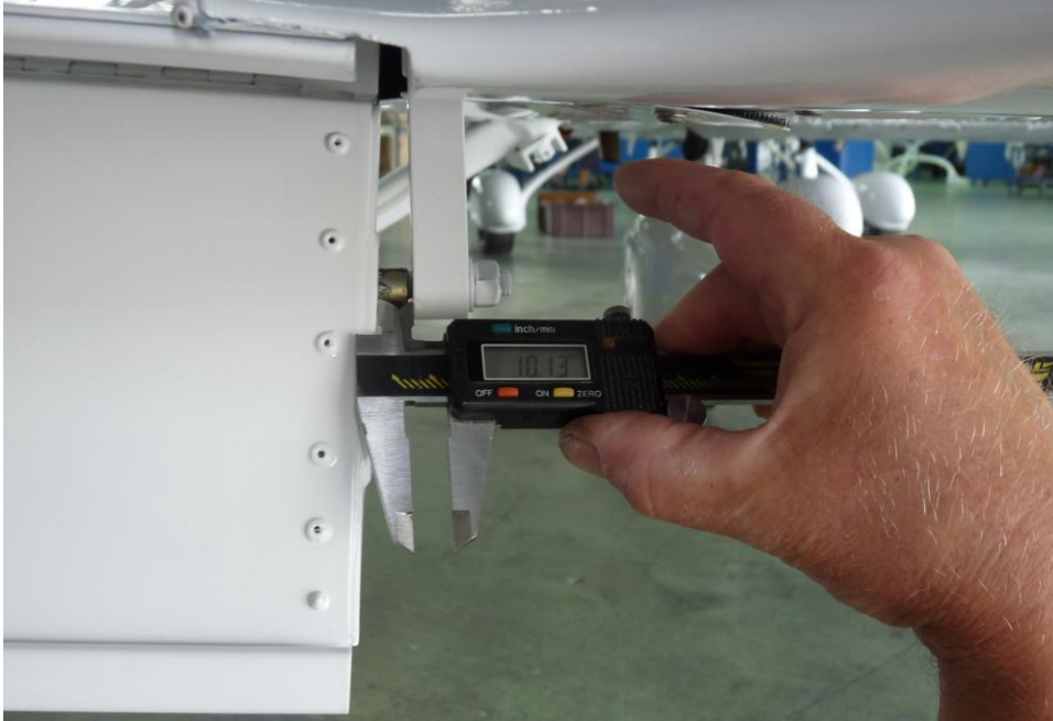
Fig. 2 – Measuring of dimension A at the left flap.
