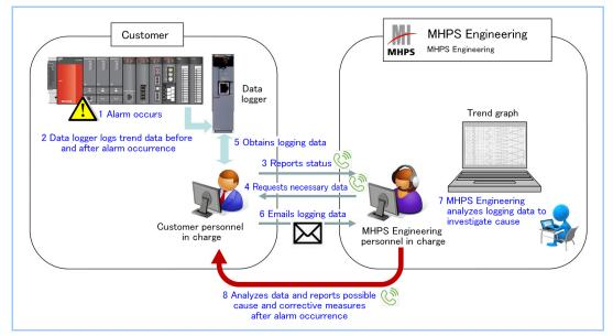
Figure 8 Conventional handling process of MHPS Engineering for alarm event
