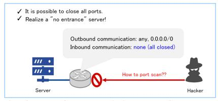
Figure 2 Feature of secure communication technology (2): All inbound communication ports of connection destination machines can be closed
