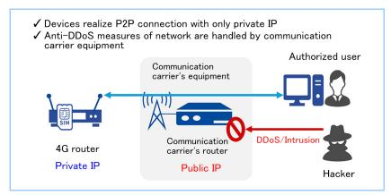
Figure 1 Feature of secure communication technology (1): No public IP used for P2P (Pier-to-Pier) connection
