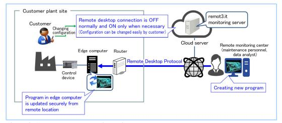
Figure 6 Access to remote machines using remote desktop
