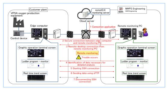
Figure 9 Outline of VPSA remote monitoring service system and secure connection process
