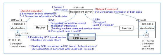
Figure 3 Secure communication mechanism combining NAT traversal and unique encryption technology
