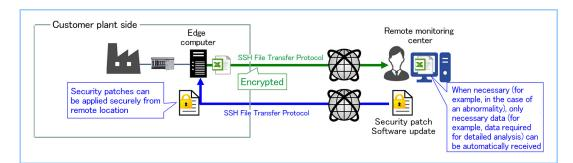
Figure 7 Secure file transmission (including automatic connection, transmission and disconnection functions in the case of an event)
