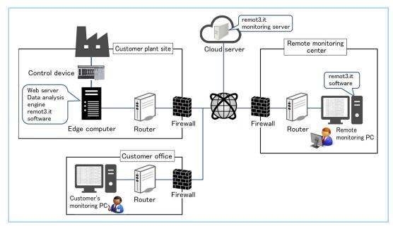
Figure 4 Remote monitoring service system using edge computing
