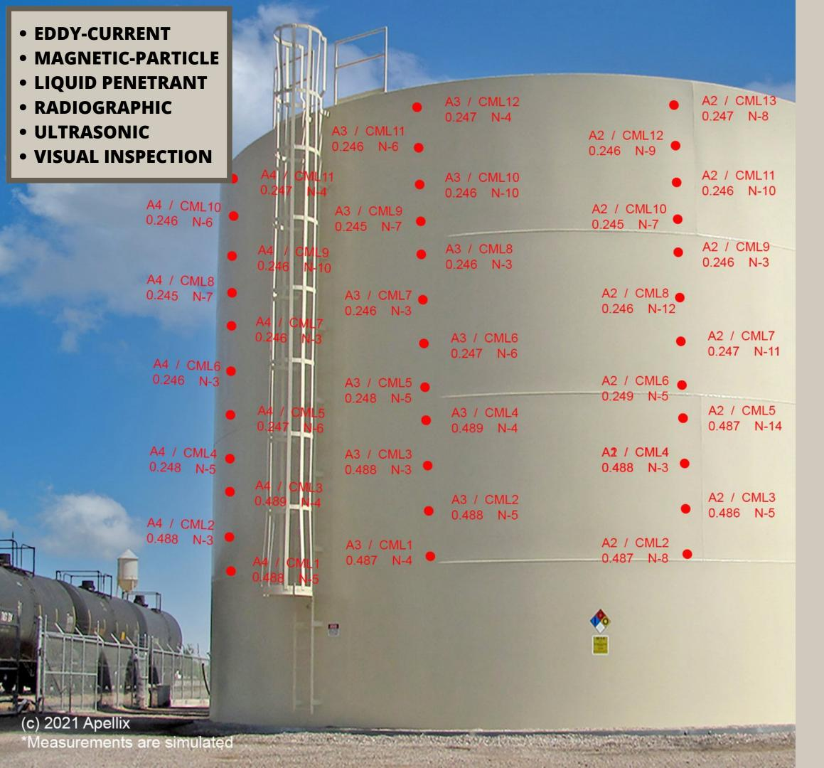
The Opus X4 NDE systems **autonomously collect data** similar to what is shown here. In this example, the aircraft pilot flies up to the structure engages the software and the aircraft then takes readings in a vertical line approximately every .25 meters (10") stopping at the top of the tank and waiting for the pilot to manually fly it to the next location and reengage the software.
