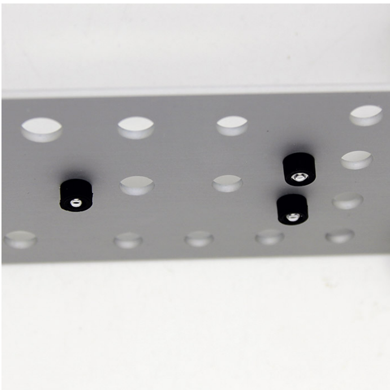
28 – Insert LED light pipes and retainer clips
