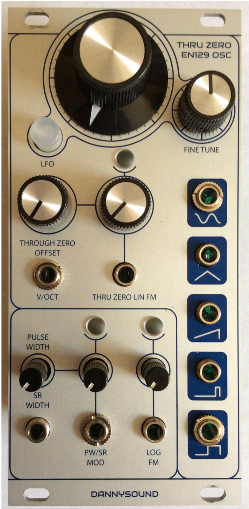
33 – Add knobs and solder one ground tab of each pot.
