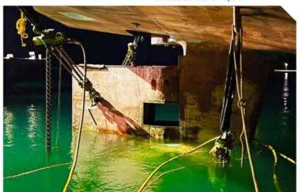
This enabled repairs to the rudder blade and its associated equipment onboard to be carried out simultaneously, so the work was able to be completed in quick succession.
