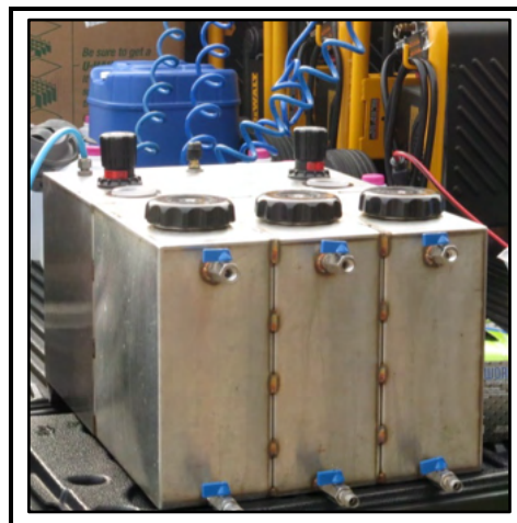
Figure 1. Dry-fog application system.
