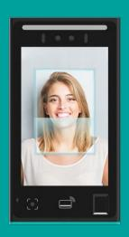
Secure. Convenient. Integrated. The Aratek BA8300 is a compact and powerful IP65 rated facial recognition terminal with multi-factor authentication capability that allows facial ID authentication, fingerprint recognition, barcode scanning and RFID card reading at once. The BA8300 facial recognition terminal serves as the ultimate digital identity workhorse, delivering unparalleled results. It provides a versatile access control and time attendance solution that meets the demands of modern times.
