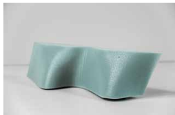
Sample wall geometry - one of two components, which are individually cut by the robot and glued to comprise one complete wall element
