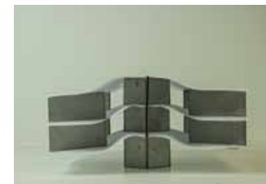
Structural tests – without a system to transmit the weight of the walls to the core, the walls sack down
