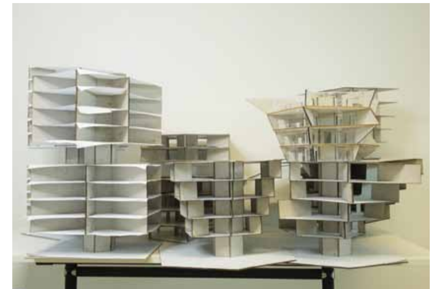
Structural tests – without a system to transmit the weight of the walls to the core, the walls sack down
