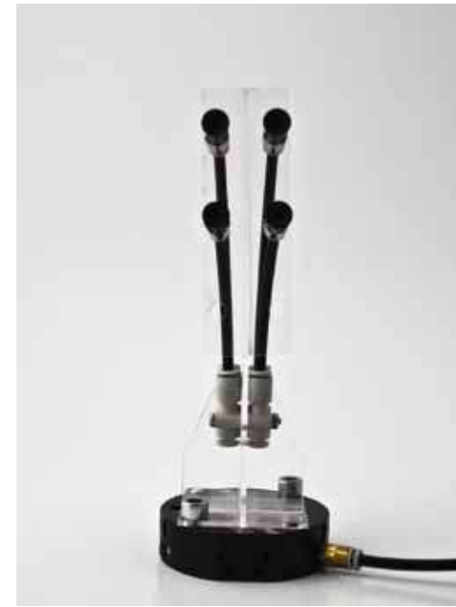
The grippers angles are optimised for picking and placing MDF sheet material
