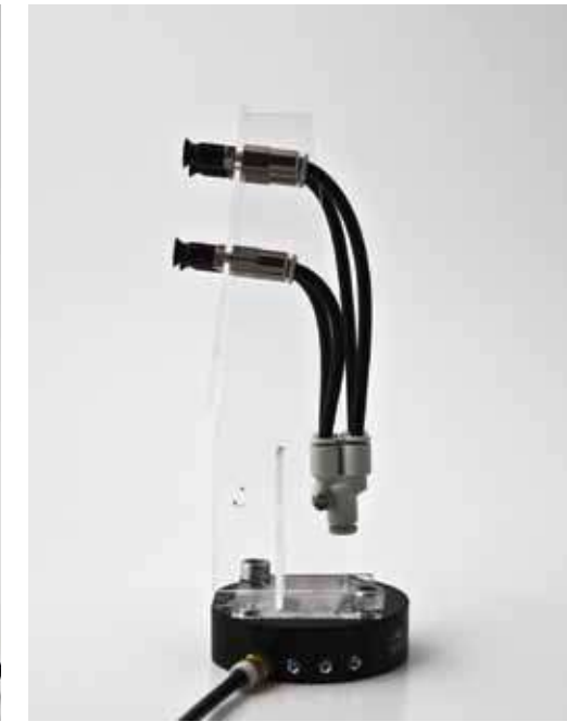
The grippers angles are optimised for picking and placing MDF sheet material
