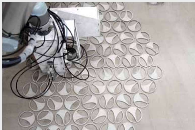
Component placing at the start of the robotic assembly process
