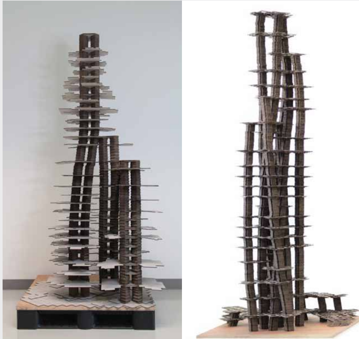
The first series of experiments with separate cores: an earlier version (left side) consisted out of stacked rectangles, which allowed horizontal floor slabs of various shapes to be interlocked. A later version (right side) demonstrates how a similar set of elements can be both vertically stacked and cantilever out to provide horizontal planes
