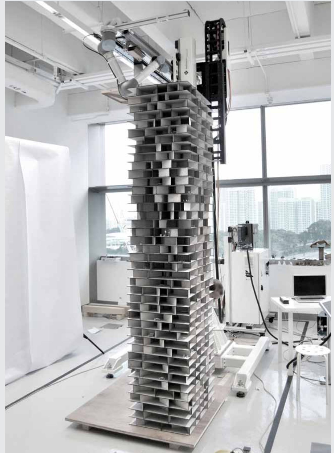
First interim tower in 1:50 scale that is assembled from folded sheets as load bearing walls
