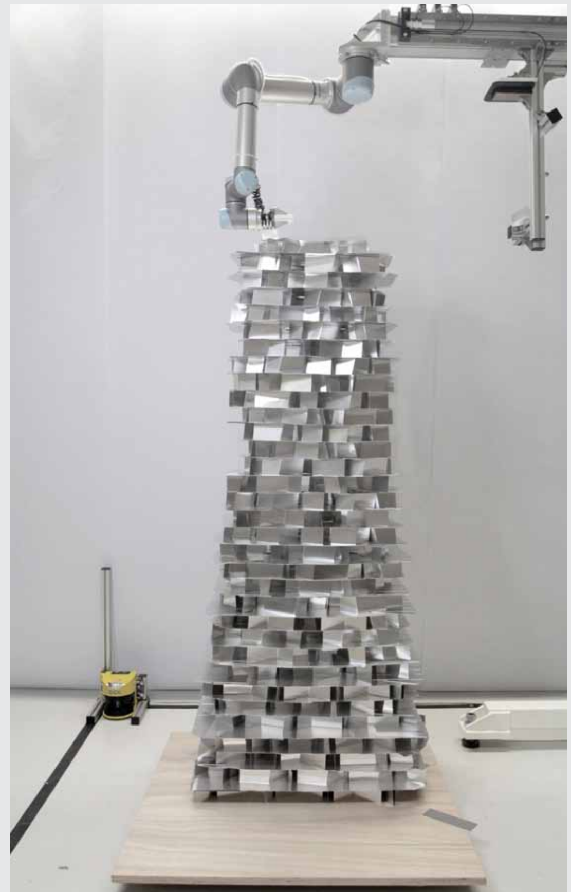
Preliminary tower before completion. The robot picks flat aluminium sheets, and folds them to specific angles before placing them
