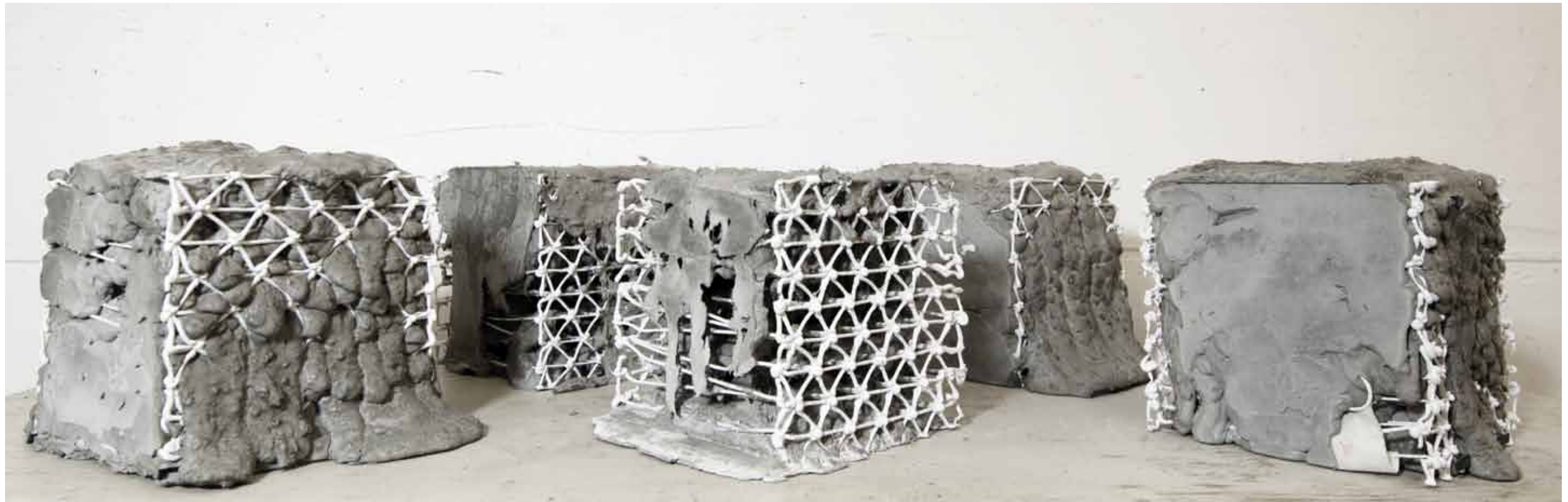
Fig. 14 Test cubes after curing - the samples have not been vibrated. The samples using a less viscous concrete display a certain degree of honeycombing and the inclusion of voids
