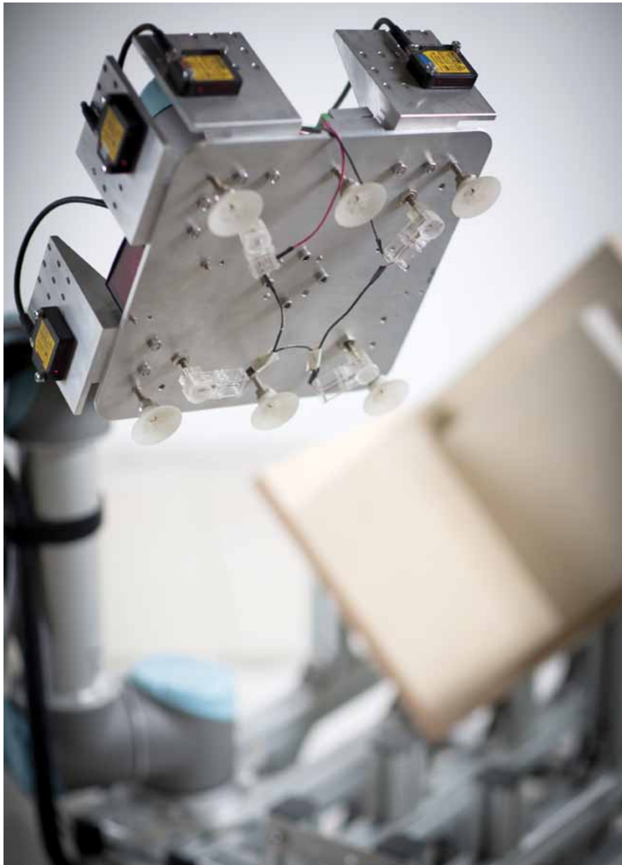
Fig. 03 The custom end-effector
