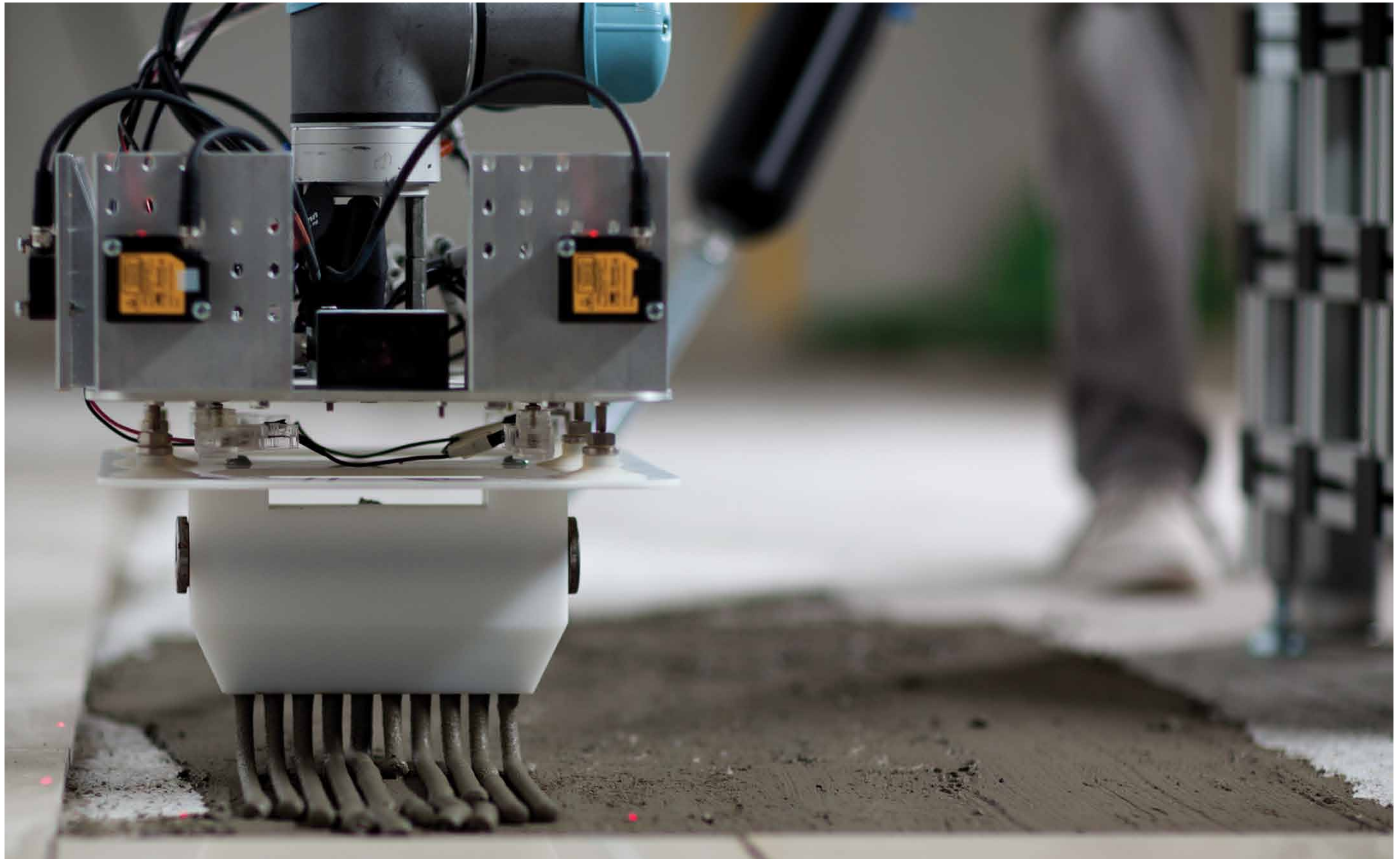
Fig. 07 The mock-up prototype of the automated adhesive applicator, the first generation of a special nozzle and extrusion tool that can be operated by the robotic arm
