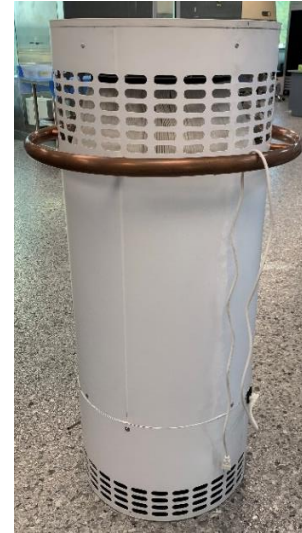
Figure 1: Violett L Device: The Violett L device is a standalone air purification system equipped with HEPA filtration and a photocatalytic vortex chamber that uses UV-C emitters. The pictured device has a prototype enclosure with production working components.
