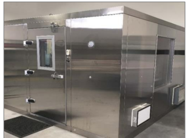
Figure 2: Stainless Steel Bioaerosol Test Chamber used for all Violett L Testing. The chamber is equipped with HEPA filtered air (in/out), multiple bio aerosol sampling ports, decontamination, and pressure balance. Exterior picture.
