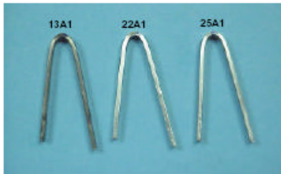
Figure 5 – General view of the normal coupons identified as 13A1, 22A1, 25A1 after the bend test following ASTM A262 Practice E as a guideline; the test coupons displayed no evidence of fissures and cracks on bending
