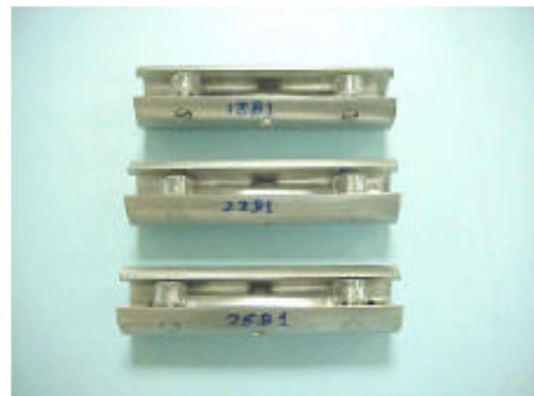
Figure 21 – General view of the bent coupons after stressing in the bending fixtures; the view presented is before exposure to the down hole environment; the bending fixtures are identified as 13B1, 22B1, 25B1
