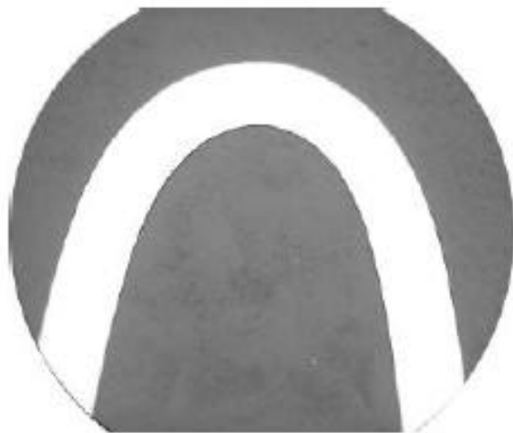
Figure 9 – Close view of the polished section of the normal coupon identified as 25A1; the section display no evidence of cracks
