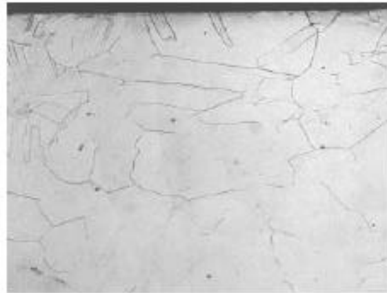
Figure 19 – General microstructure of the normal coupon identified as 25A1 away from the bend location displays a relatively equiaxed austenitic grain structure, which is representative of the original material; Original magnification – 100x
