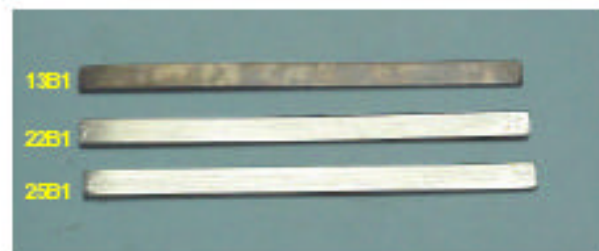
Figure 23 – General view of the bent coupons identified as 13B1, 22B1, 25B1 after exposure to the down hole environment in the stressed condition; the coupons were removed from the fixtures (see Figure 22); note coupon identified as 13B1 displays discoloration whereas the other two coupons display original bright metallic luster
