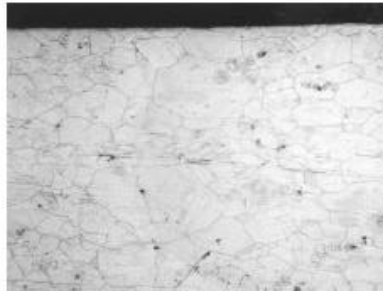
Figure 16 – General microstructure of the normal coupon identified as 22A1 away from the bend location displays a relatively equiaxed austenitic grain structure, which is representative of the original material; Original magnification – 100x
