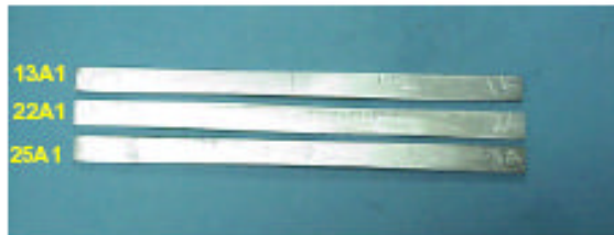
Figure 3 – General view of the normal coupons identified as 13A1, 22A1, 25A1 before exposure to the down hole environment; note all the samples display the normal metallic luster expected in the as-machined condition
