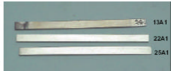
Figure 4 – General view of the normal coupons identified as 13A1, 22A1, 25A1 after exposure to the down hole environment; note coupon identified as 13A1 displays discoloration whereas other two coupons display the original bright metallic luster
