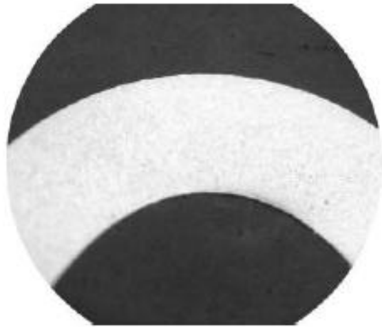
Figure 11 – Stereomicroscopic view of the etched metallographic section from the bend location of the normal coupon identified as 13A1
