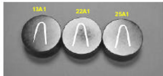
Figure 6 – Polished microsections from the bend/deformed locations of the normal coupons 13A1, 22A1 and 25A1
