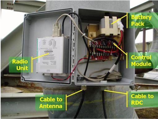
Figure 4 - Remote Monitoring Components
