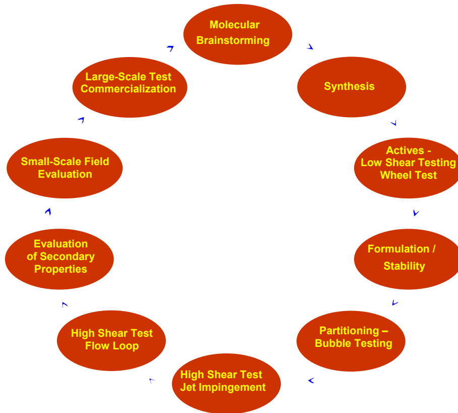
Figure 2 - Corrosion Inhibitor Development Process
