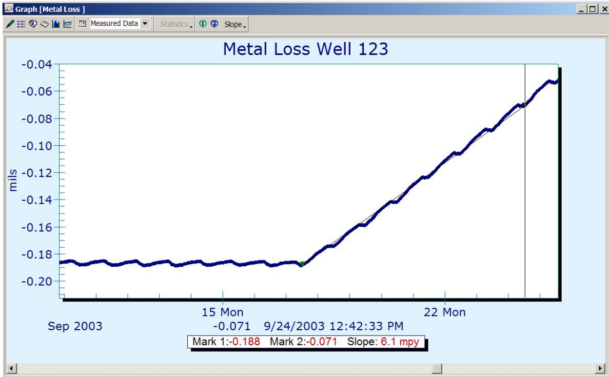
Figure 12 Corrosion Upset from Microcor Transmitter on Upstream Gas System
